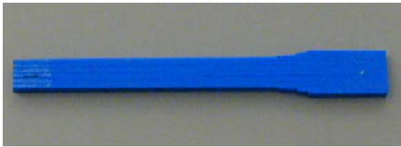
Figure 3.4 Trouble with stress concentration - 3" radius actually infinitely small resulting in premature shearing at left end of sample.
