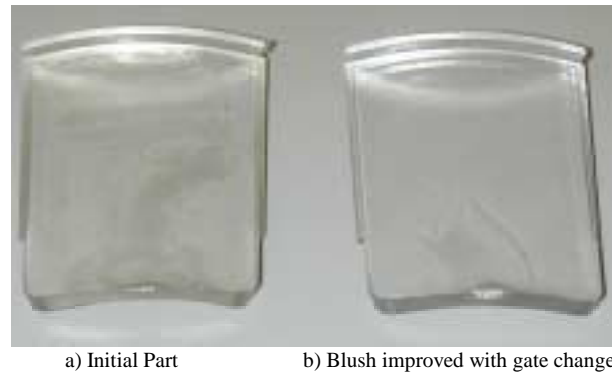
Figure 20: Blush Marks on Windows
