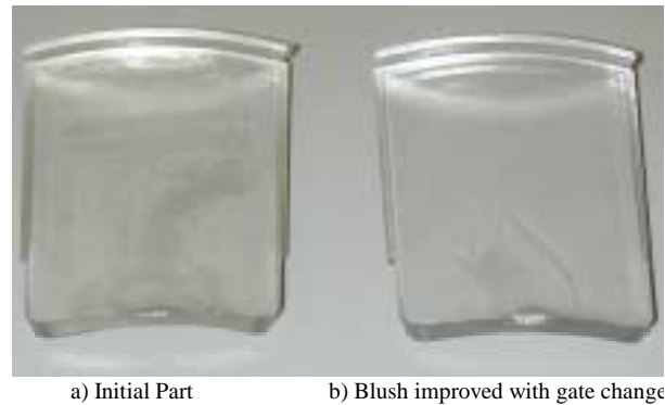
Figure 20: Blush Marks on Windows
