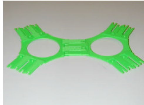
Figure 1: FDM prototype of the Triconnector
