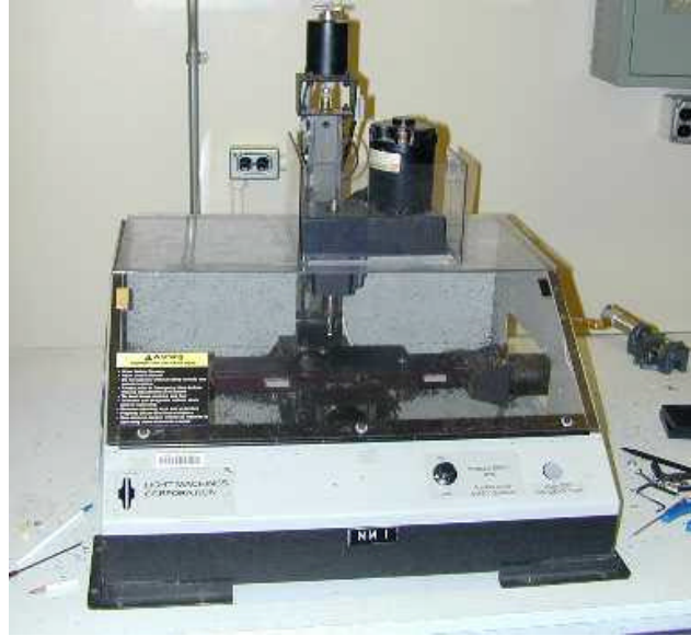
Figure 1.1: Spectra Light Mill Used in Project
