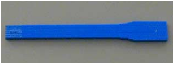
Figure 3.4 Trouble with stress concentration - 3" radius actually infinitely small.
