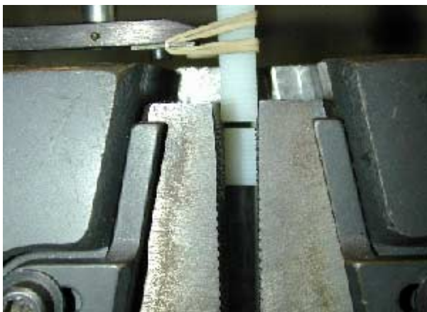
Figure A.5. Tangential (2) failure total rupture at grip.
