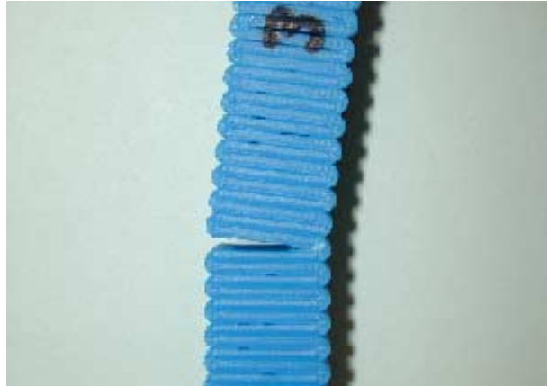
Figure A.2. Tangential (2) failure: rupture of bond between beads.
